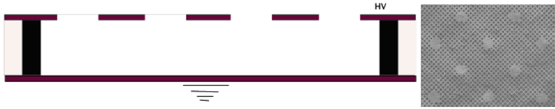
Figure 2. Left: Kapton pillars are created with a step of about 500 microns; Right: photo of a mesh with copper spots used to protect the polyimide bellow during etching in order to form the pillars.
